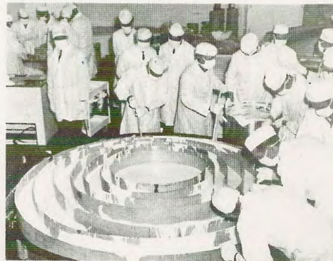
FORMING A SPACECRAFT'S HEAT SHIELD
