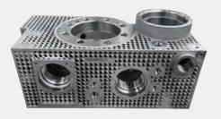
By using AM techniques, Marotta produced a direct replacement of a chilled water valve with delta qualification which previously had a 29-week lead time for its traditional sand-cast brass body. Marotta's engineering team replaced the brass valve body with a requalified version produced via Laser Powder Bed Fusion (LPBF) using Inconel 625, a corrosion-resistant nickel superalloy.
