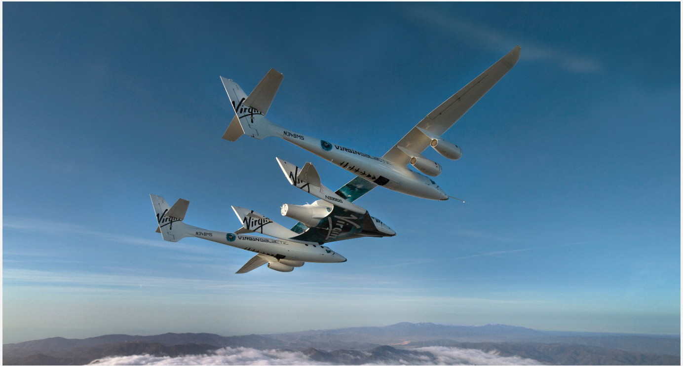
Virgin Galactic’s “captive carry” flight test, during which VSS Unity remained mated to the firm’s WhiteKnightTwo mothership (VMS Eve) for the entire flight. Marotta is proud to partner with Virgin Galactic on this program. Photo courtesy of Virgin Galactic.
